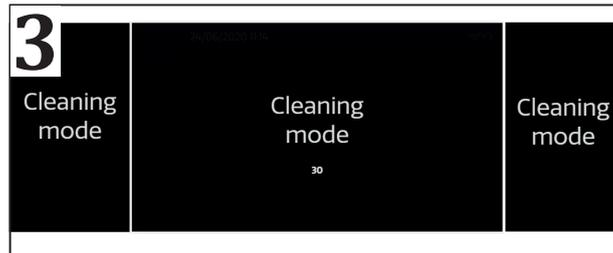
For 30" the capacitive displays are disabled. After completion the displays will show the work screen again.
