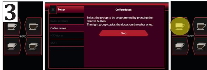
Attach the portafilter with the coffee to the 1st, 2nd or 3rd group starting from the right and press the one short coffee button to start the delivery.
