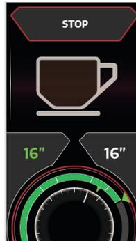
**During the following delivery, if the coffee extraction is within the range of time stored by the service during the installation phase +/- the selected tolerance, the progressive bar will be green. Otherwise, in case incorrect delivery time, it will turn red.**
