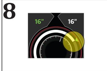
A progressive white circular bar will show if the preset time has been reached (green triangle). If it turns red, it means that the extraction time is shorter or longer than the programmed one.
