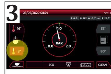
Or press the button on the bottom left hand side (O, page 4) to deliver mixed hot water. The delivery stops at the end of the time programmed during the installation.
