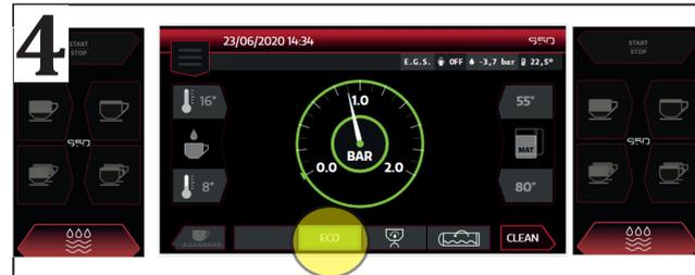
4 The boiler temperature reaches 85°C. Press the ECO button again to deactivate the ECONOMY mode. In about 15 minutes the machine will be ready to work.
