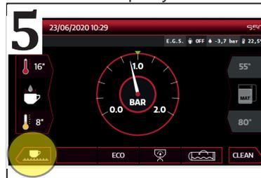
Push the same button to turn off the cup warmer heating element.
