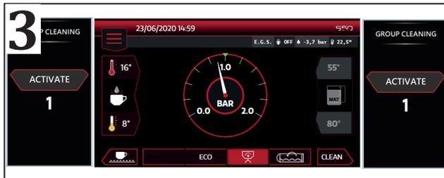
The GROUP CLEANING cycle consists of 5 seconds of water delivery from the selected group, followed by 5 seconds of STOP, thus allowing the use of the brush to clean the group showers.
