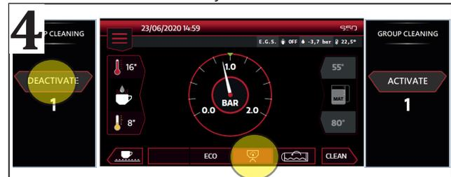
Press the DEACTIVATE button to stop the cleaning cycle. Press the GROUP CLEANING button again to return to the work screen.
