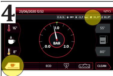
With the cup warmer turned on, the temperature of the cup tray is shown on the status bar.
