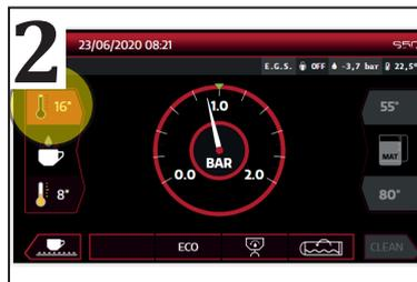
Press the button on the top left hand side (P, page 4) to deliver hot water. The delivery stops at the end of the time programmed during the installation.
