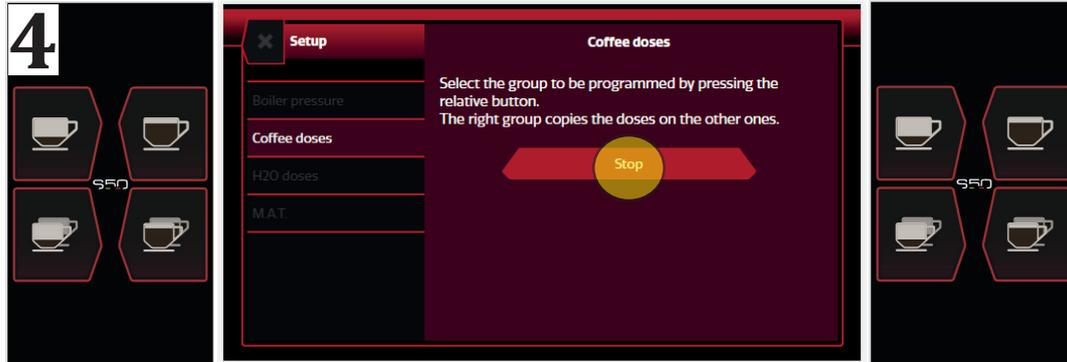
Once the desired amount of coffee in the cup is reached, press the same button to stop the coffee delivery. Repeat the same procedure with the other buttons. Press "Stop" at the end. The group on the right copies the doses on the other groups. In case you want to program the 2<sup>nd</sup> or 3<sup>rd</sup> group differently from the others, program the dose buttons of the other groups separately.
