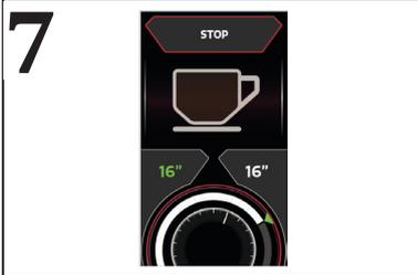
In case of preset doses, the display shows the programmed time (in green on the left) and the real extraction time (in white on the right).
